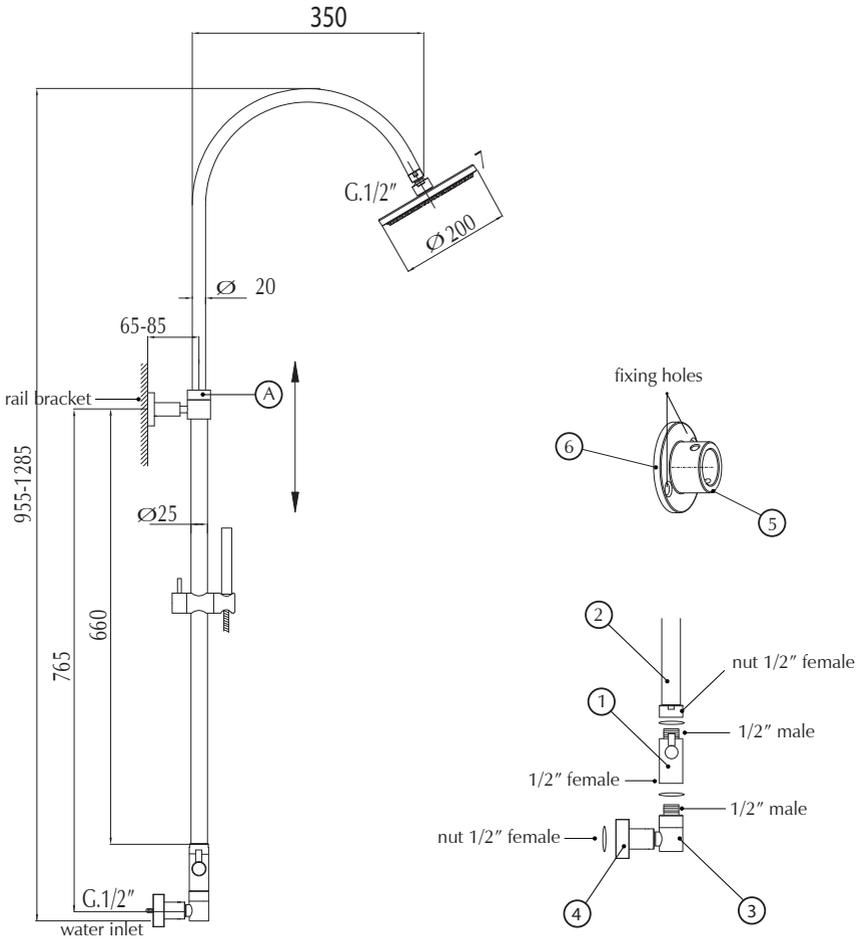
**NOTE: Riser pipework MUST not be cut.**
